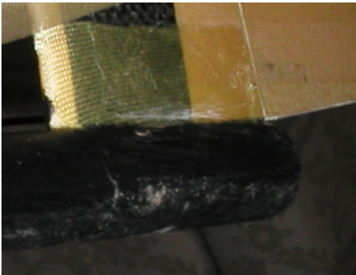
Figure 15 Kevlar wrap around boom and Vertical stab
