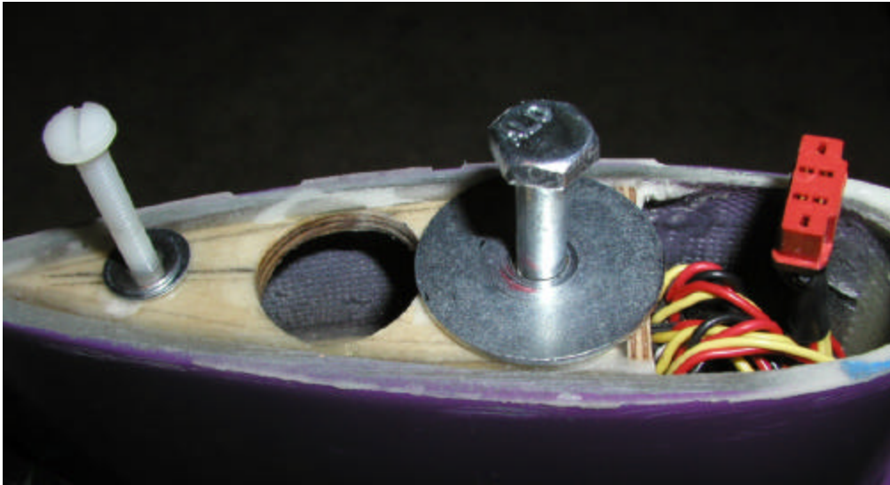
Figure 8 Wing Pylon with RX in place
