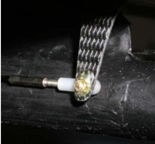
Figure 16 Elevator Control horn with ball joint & pushrod
