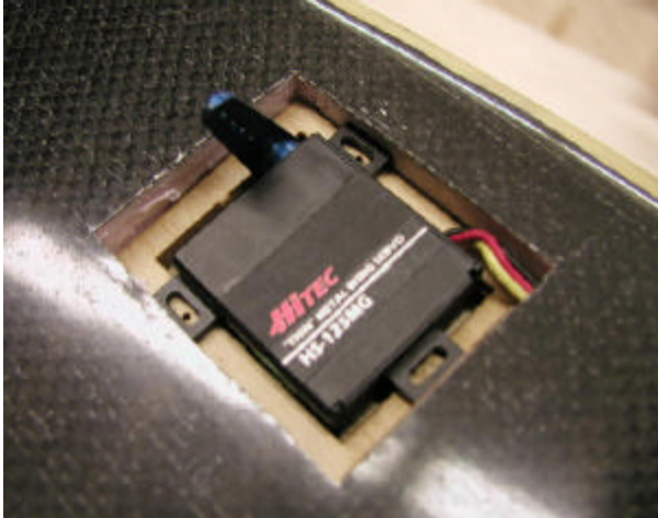
Figure 24 Aileron Wing servo installation HS5125
