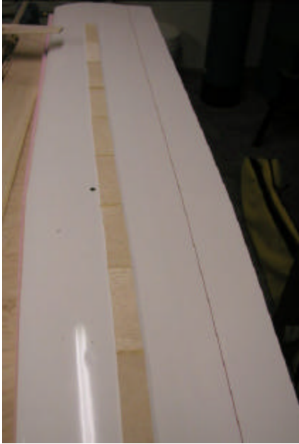
Figure 10 Pushrod support balsa laid on wing
