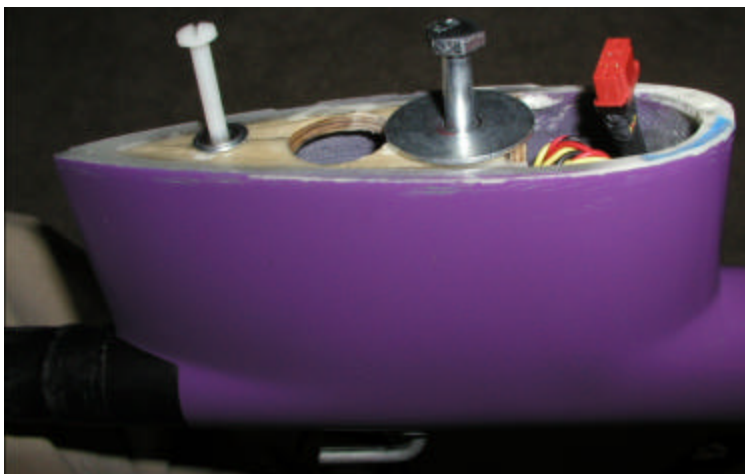
Figure 9 Wing pylon complete, Note Epoxy skim to match wing shape to pylon
