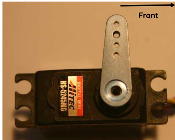
4. Remove the servo arm and rotate it 20 or 30 degrees toward the rear of the wing.
