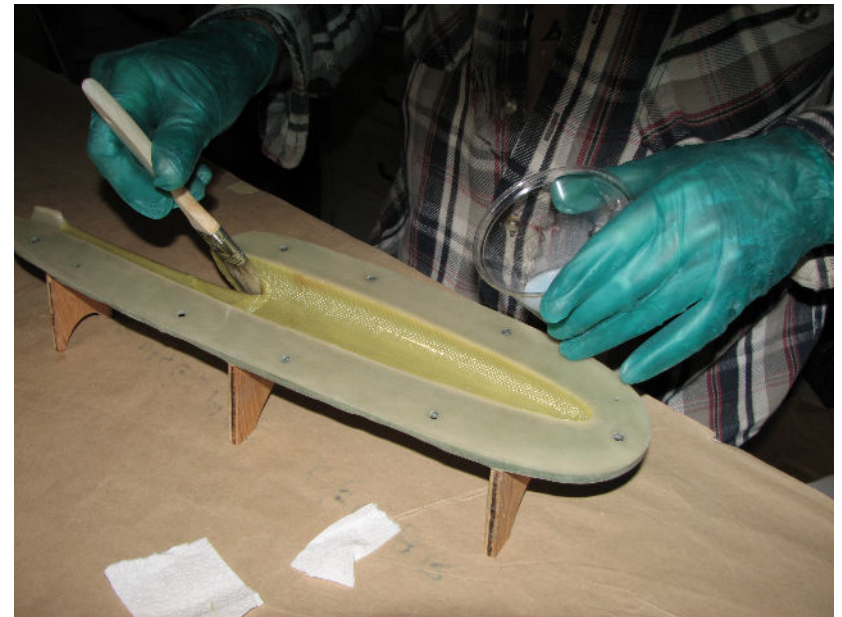
Left: Patch in place and resin applied. Right: The first layer is trimmed flush to the mold flange and allowed to partially cure. A layer of resin is brushed into the mold before the second layer of cloth.
