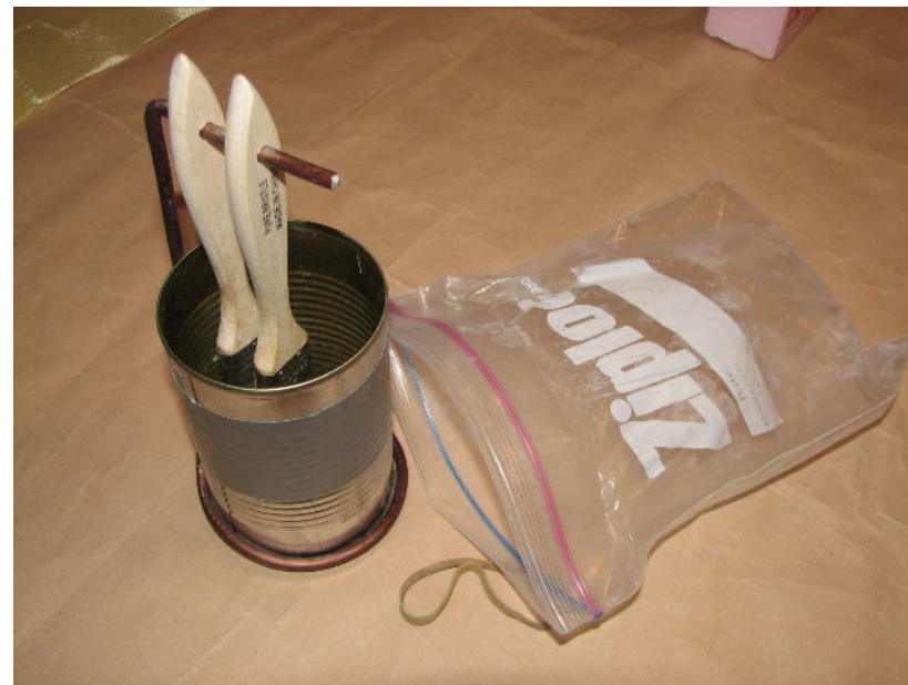
Right: Brushes are cleaned and stored in MEK 96.
