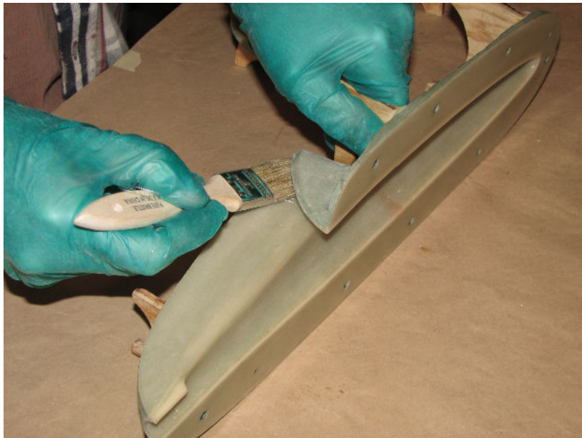
Left: MGS epoxy, with colloidal silica added, is painted over mold surface.
