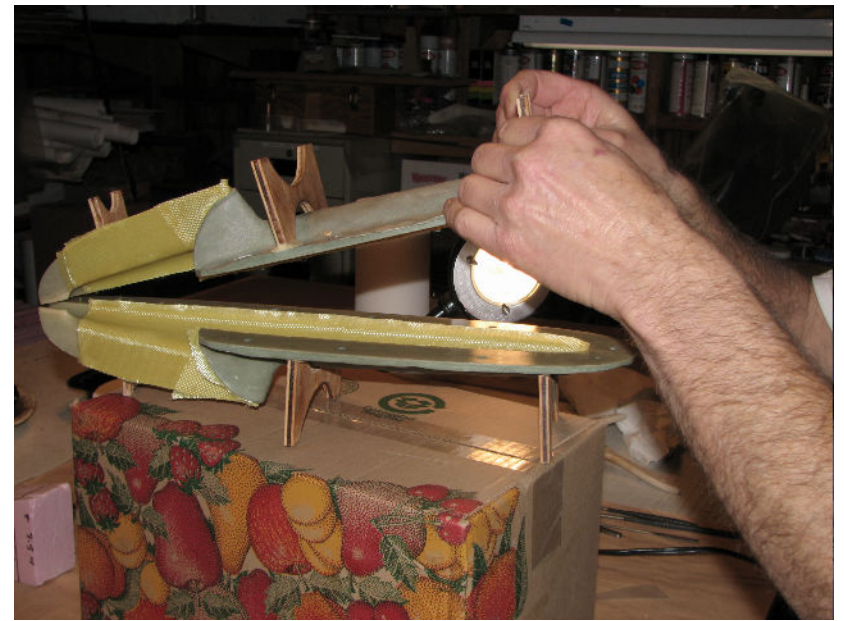
Right: The mold halves are positioned, with good lighting, for joining.
