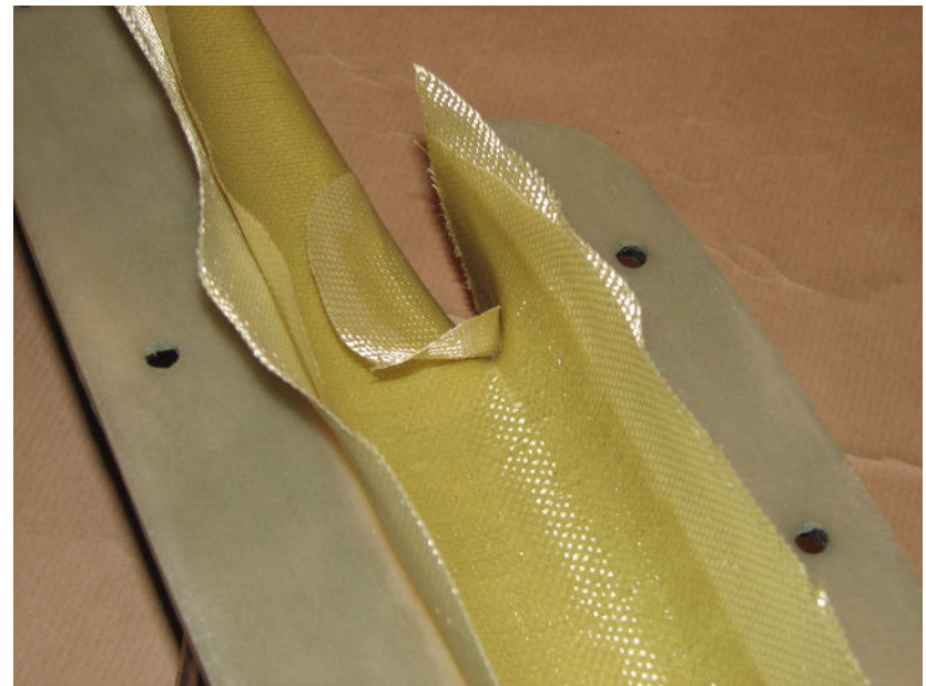
Left: The second layer of cloth is placed and resin stippled through. The second layer is placed with the weave on a bias to the pod longitudinal axis. A third layer of cloth is then added. The first and third layers have weave parallel to the longitudinal axis of the pod. Right: A second patch, with weave biased, is added. A small amount of resin is brushed around the patch cutout area.
