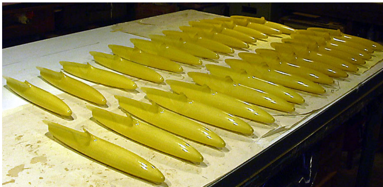
Above: Fuselage pods, trimmed with Lexan scissors, prior to packaging.
