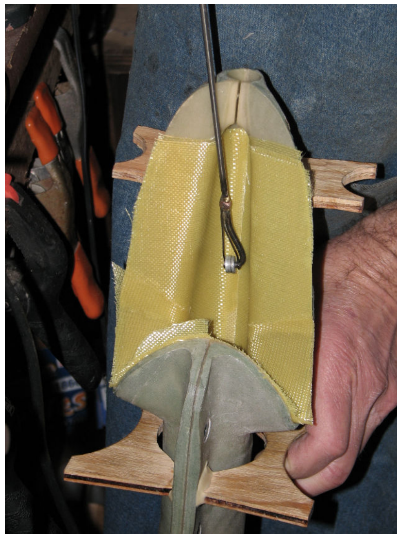
Right: Close-up of seam rolling process.
