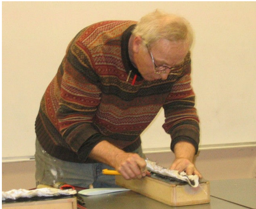
Epoxy partially hardened, Stephen trims off the extra cloth.
