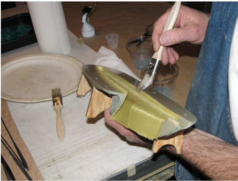
Left: A small amount of resin is applied along the seam prior to joining the two halves.
