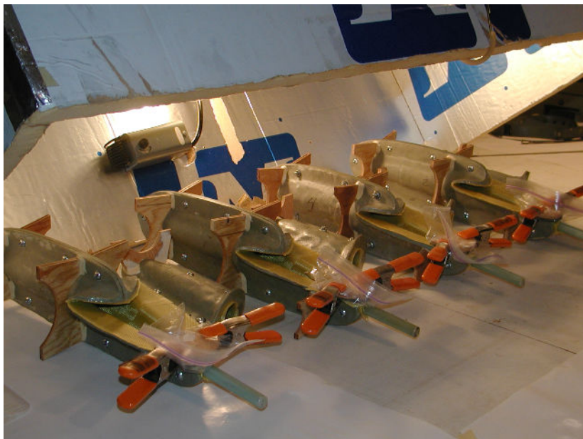
Left: Molds are placed in a heat box and cured overnight at 85 degrees Fahrenheit.
