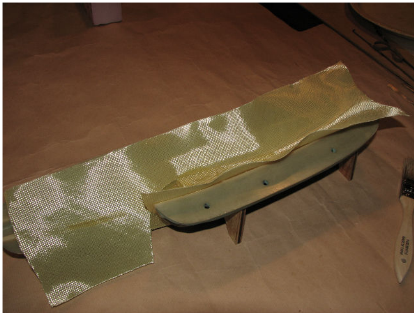
Left: The second layer of cloth is placed and resin stippled through. The second layer is placed with the weave on a bias to the pod longitudinal axis. A third layer of cloth is then added. The first and third layers have weave parallel to the longitudinal axis of the pod. Right: A second patch, with weave biased, is added. A small amount of resin is brushed around the patch cutout area.
