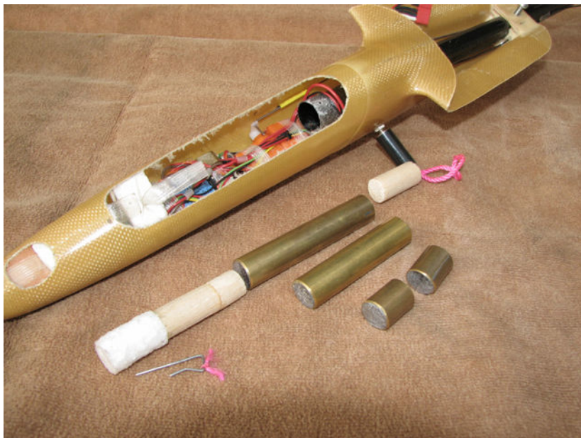
Left: Ballast weight arrangement. Standard ballast consists of three concentric weights.
