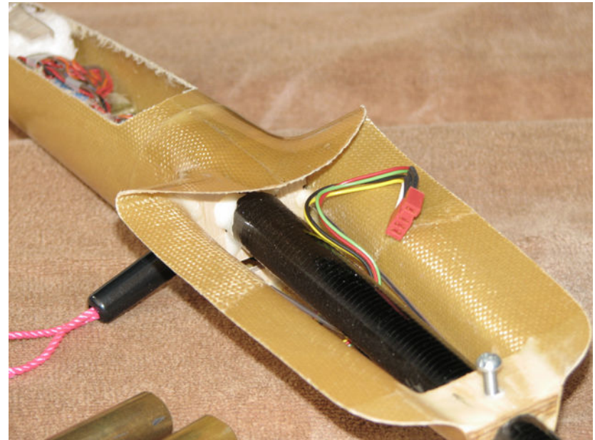
Right: Fuselage pod detail showing carbon tube extended forward to house ballast.
