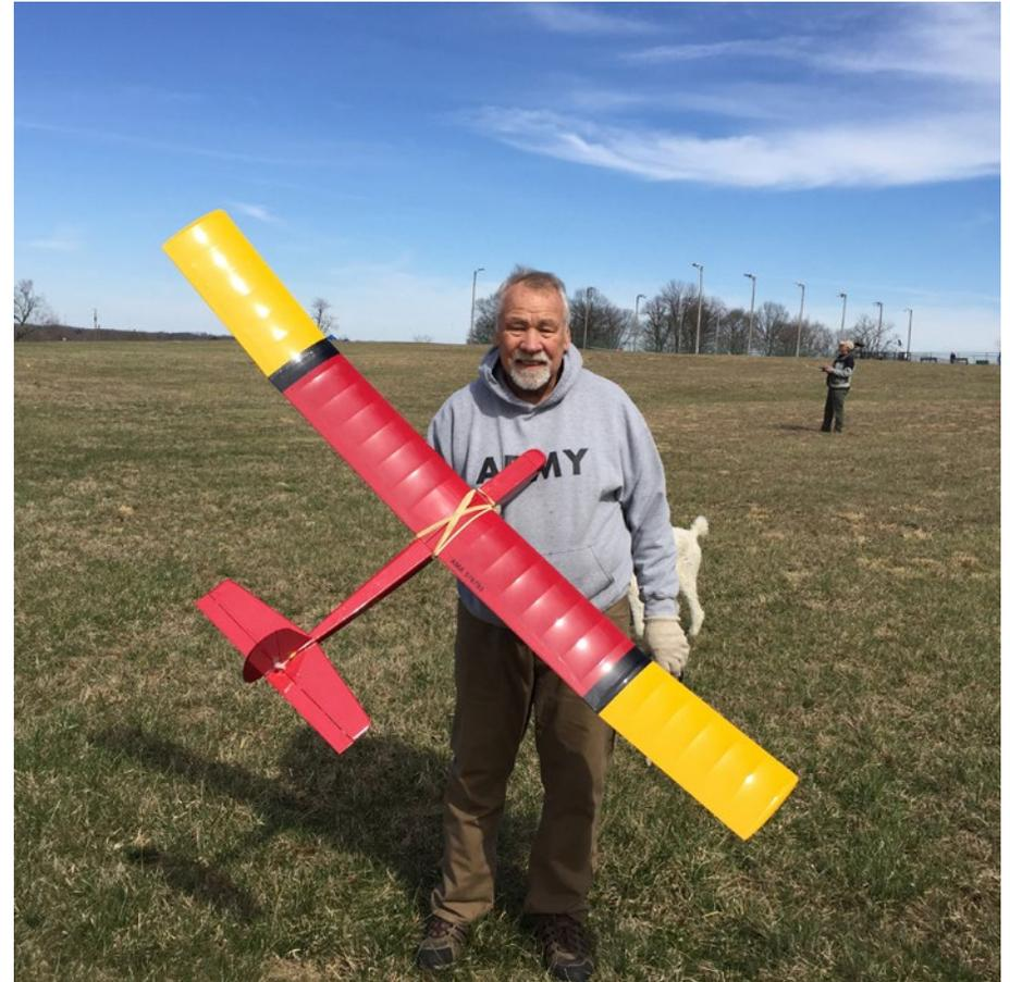
*Gordy and his Airtronics Square Soar. It was created by Lee Renaud to fill in the bottom end of their product line. Totally competitive, believe it or not, despite having a span of just 70". Simple, cheap, one rib size and shape for the whole wing... turned out to be a really good sailplane! I got this one at a Dayton Swap meet. First flight off a F3RES spec high start in very cold air was 20 mins. You can see it fly if you visit <<https://youtu.be/FgjZEbpFM0o>>.*
