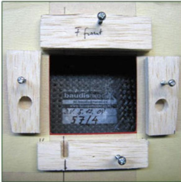
The blocks prepared for installation. These are 3/16" balsa, which suffices for these stiff carbon wing skins. For more flexible skins, consider using thicker balsa and/or pieces with vertical grain.
