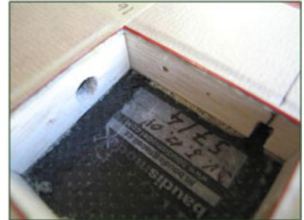
This "box" ties the top and bottom wing skins together to form a rigid pocket which will not flex under load. I used very little PU glue which foams slightly and forms a strong and light-weight build.
