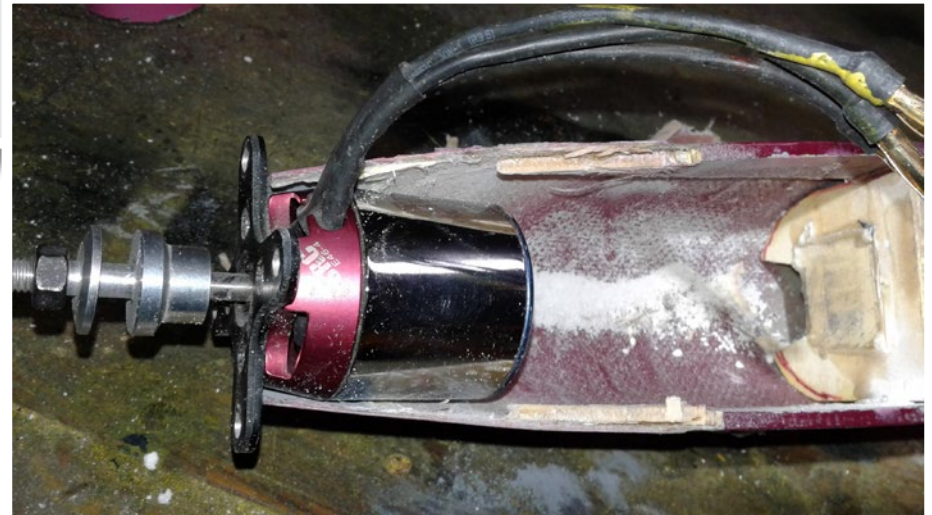
Fitting the eFlite Carbon Cub motor.
