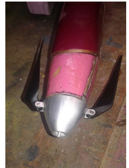
Motor mounted and nose wrapped with \frac{3}{4} oz. 'glass.
