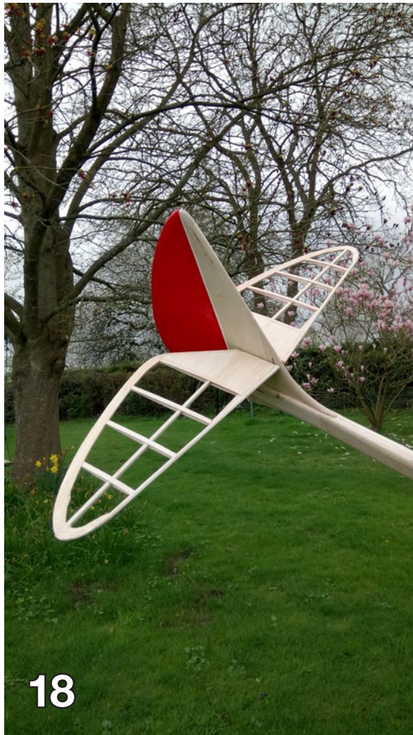
(18) All moving tailplane and rudder are similar built-up construction.
