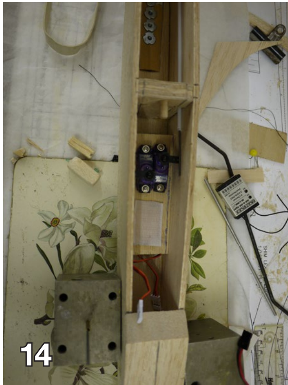
14 - Rudder and Elevator servos and receiver tray is under canopy for easy access, leave room to ensure your chosen battery can be slid down the nose.
