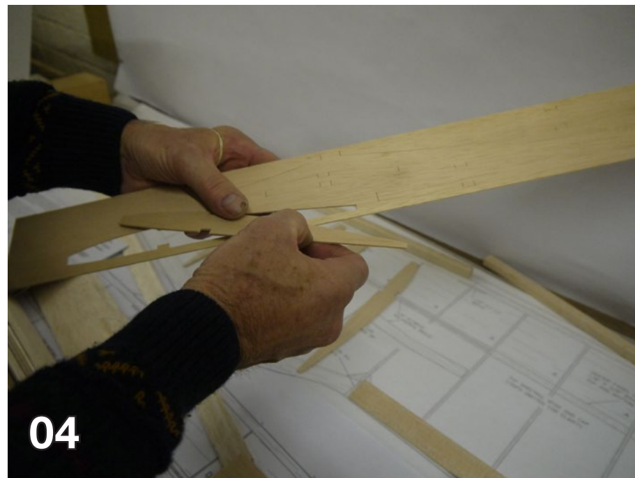
(04) Shaped parts are die cut and push out easily.
