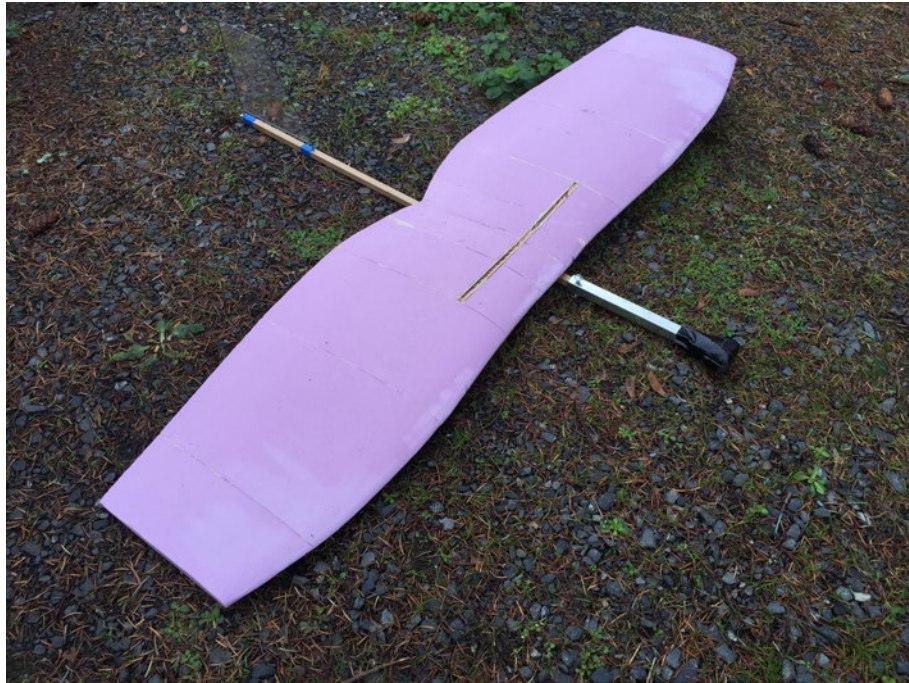
Styrofoam wing without tip feathers to check CG.
