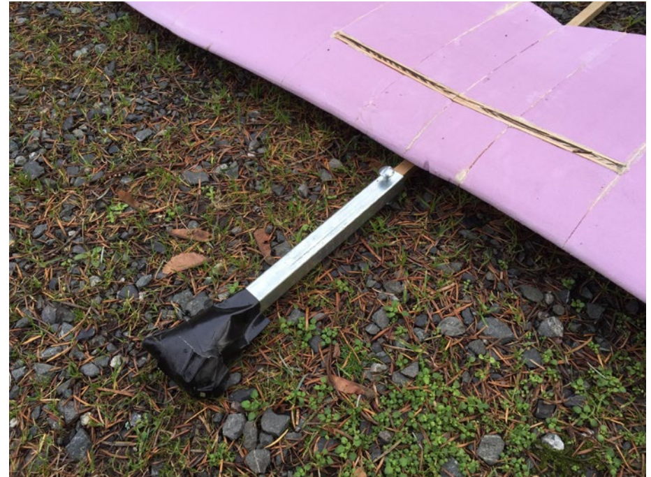
CG varied by moving square tube along "fuselage" nose.
