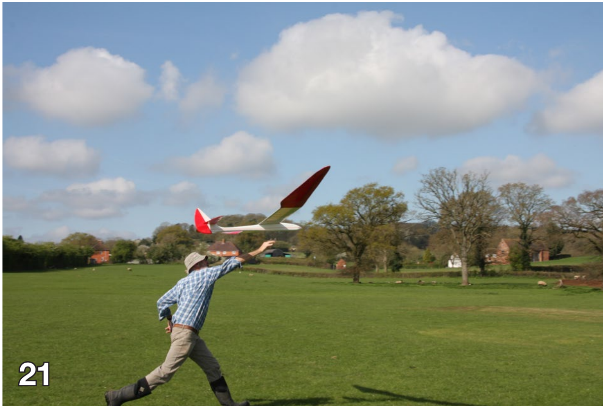
(21) Trial hand launch to check out centre of gravity and trims.
