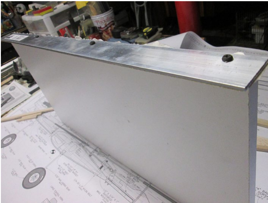
With the base on its edge, you can see how the metal sheet is attached with three screws.
