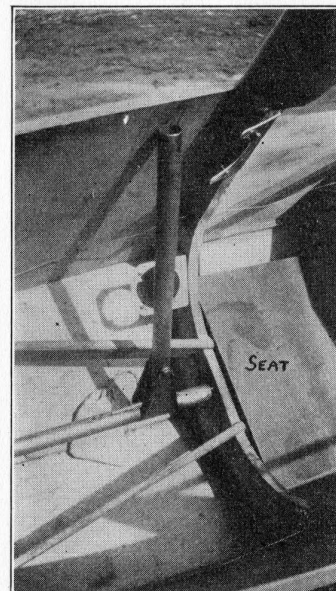
Plate XXXV. Interior of Prüfling Cockpit Showing Seat and Stick, and Instrument Brackets
