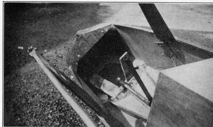
Plate XXXIV. The Prüfling Cockpit with Cover Removed, Showing the Stick and Rudder Pedals
